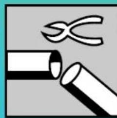
Only cut pipes with sharp cutters.
