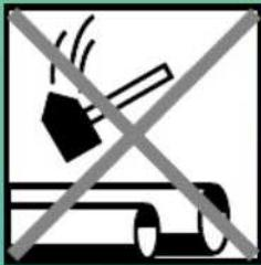
Avoid sharp impacts and strokes to the pipes, especially at low temperatures. Do not throw when unloading. Protect pipes from falling objects.
