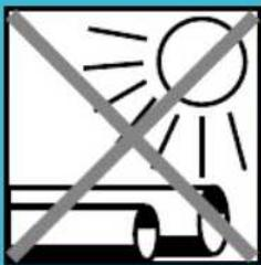
Do not expose pipes to UV radiation for extended periods of time.
