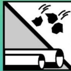
Put down pipes or pipe bundles carefully. Cover pipes in areas of falling rocks, etc.
