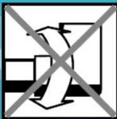
During polyfusion welding, do not twist the pipe or fitting; push the pipe and fitting joint together in a straight manner.
